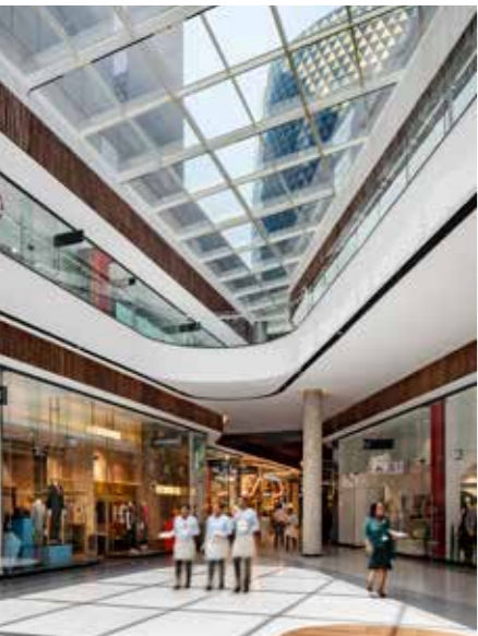
Left: Overhead skylights in the retail areas help to flood the interiors with natural light and blur the distinction between interior space and exterior urban environment.
